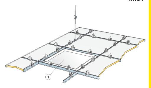
1. Connect Inspection hatch C3 (600x600/1200x600)
